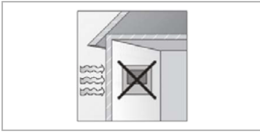
Fig. 5: Installation site - Exterior wall
