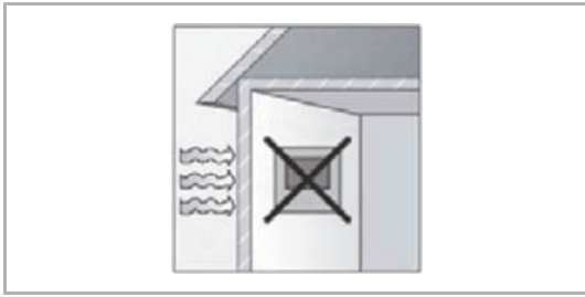
Fig. 7: Installation site - Exterior wall
