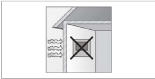
Fig. 5: Installation site - Exterior wall
